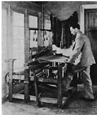
Demonstrating the Flying Shuttle on the Loom. There Are No Really Efficient Domestic Looms on the Market. The Flying Shuttle Was Added to This Loom on the Homestead. With This Attachment, a Yard of Cloth Is Readily Woven in an Hour. The Suit Worn by the Demonstrator Was a Hand-spun Twill, Woven on This Loom and Made-up by a Local Tailor.
